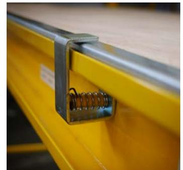
Steel edge banding protects all four sides of the exterior-grade plywood work platform without using rivets, screws or staples. Hand holds on each side provide ease in handling. Platform is held in place with spring-loaded retaining clips.
