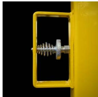
User friendly squeeze-lock is spring loaded to maintain the locked position at all times except when released for adjustment. A locking knurled knob is provided to prevent unintentional release. Additional snap pin is provided as a dual locked scaffold system.
