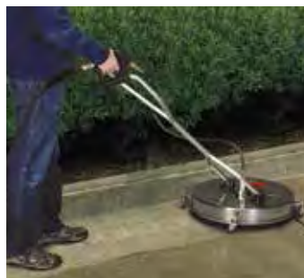
Surface Cleaner - cleans flat surfaces up to 3 times faster than a wand, and without "striping".
