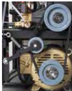
"Tru-Tite" Spring Loaded Self-Tensioning Belt
