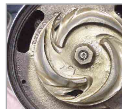
Competitor Impeller is effectively worn out.
