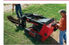
BORE DRIVE HEAD AND ROD & REAMER KIT (sold separately) Easily bore under driveways and sidewalks to simplify irrigation and cable installations. Working depth: 19"
