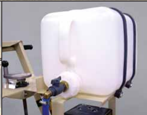
WATER TANK ASSEMBLY
