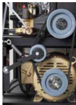
“Tru-Tite” Spring Loaded Self-Tensioning Belt
