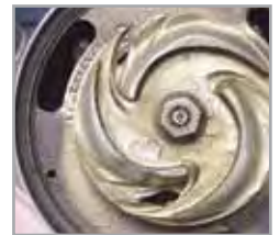
Competitor Impeller is effectively worn out.
