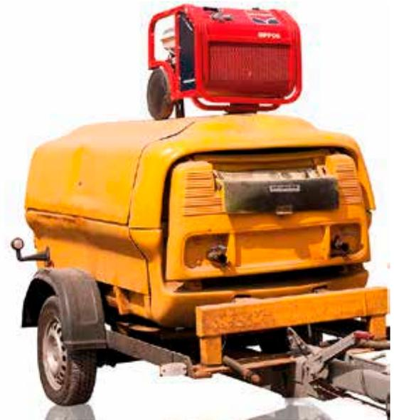
*Pictured: A hydraulic PowerPack on top of an Air Compressor, both sized to operate the same rated Breaker.*
