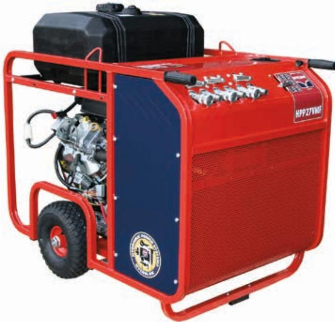
The HPP27VMF has Dual Pumps that combine for a full 16GPM flow or can be used on two different 8GPM tools. Some use a flow divided hydraulic circuit to approximate a dual even split of oil, whereby the HPP27 has two piggybacked individual pumps.
