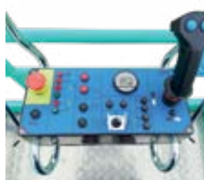
Simple and intuitive control box that can be removed from the basket for loading / unloading the machine
