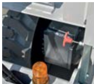
Standard manual emergency lowering device
