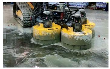
The plates for bolt-on tooling (plate p/n-200179) on the LX30 PRO and Stone Extreme have options for either 3 or 4 bolt-on segments. The hole pattens also include an option for bolt-on traps for even more options. The pin needs to be unthreaded from the universal segments and qty-3 M6 screws per segment must be used to bolt them in place.
