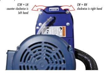
**Note: 1)** Some machines have an option to change rotation 2) Planetary machines - the planetary disc can sometimes spin opposite to the main disc
