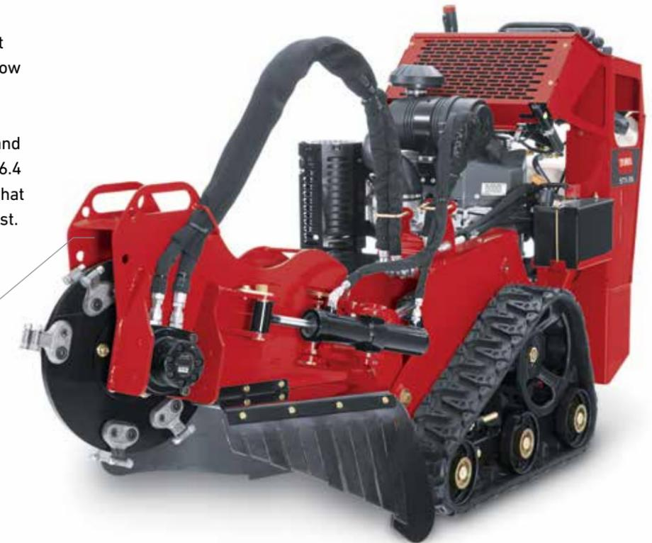
**OFFSET CUTTING HEAD** results in excellent visibility regardless of stump size.
