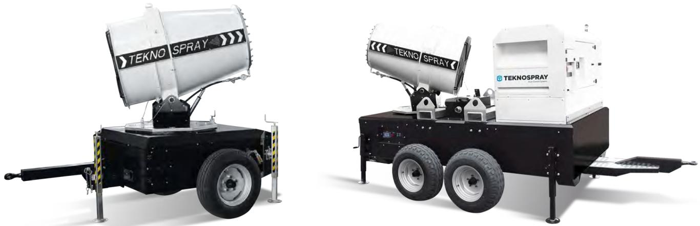
TeknoSpray, part of the Trime Group, has developed a wide range of innovative, versatile and compact dust suppression systems. Fully automatic with R.O.T. system standard - Remote control, automatic Oscillation 0-340° and electric Tilting system. Used in mines, quarries, demolition, recycling and odor removal.
